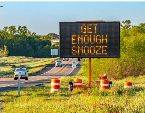
Temporary signage placement and programming (screen one)
